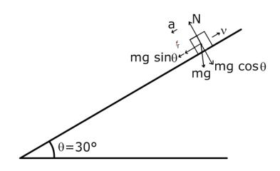
$$\begin{split} &ma = f_r + mg \sin\theta \\ &ma = \mu mg \cos\theta + mg \sin\theta \\ &a = (\mu \cos\theta + \sin\theta)g = (0.1\cos 30^\circ + \sin 30^\circ)10 \\ &= \frac{\sqrt{3}}{2} + 5 = 5.87 \text{ m/s}^2 \end{split}$$
